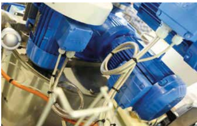
Loops along the cables trap dirt and are tough to clean, so they should be avoided in food production.
