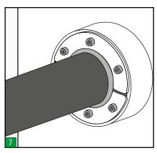
Make a visual inspection of the transit. HRST (colour code) selected match the pipe and sleeve installed, HRST is completely inserted into the sleeve, does not exist gaps between HRST and the cable/pipe.
