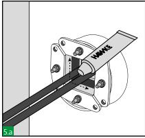
Lubricate the inside of the HRTO and all the insert and blank blocks using Hawke lubricant. Open the two front plates. (HRTO30, HRTO40 & HRTO50 front plates are fixed)
