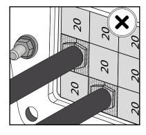
Check the correct orientation of the blocks.
