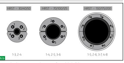
Tighten the bolts. Tightening must be done in one revolution step for each bolt following next sequence until the system is enough compressed to seal the cable/pipe.
