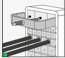
Remove endpacker nuts and front plate.
