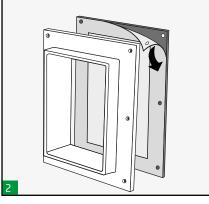
Remove the protection and stick the gasket on the aluminium frame.
