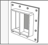
Check that Hawke Frame has been used in the installation, that it has been properly installed (welded/bolted)and that it has not mechanical or corrosion damage.
