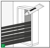
Lubricate the inside of the frame. Ensure the corners are well lubricated.
