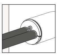
Check that all the bolts has been tightened similarly and do not exist gaps between the cable/pipe and the HRST.
