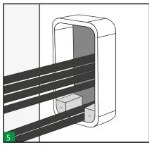
Insert HF200/R20 or HF300/R20 round corner blocks in the bottom corners of the frame.
