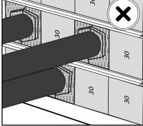
Check the correct orientation of the blocks.
