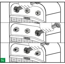
Tighten the nuts on the endpacking alternately following the above sequence to compress and complete the seal. Use a ratchet spanner for an easier installation.
