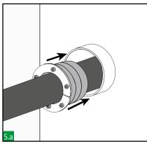
Insert the HRST into the sleeve. Check the HRST is completely inserted into the sleeve, front plates should be in contact with the sleeve.
