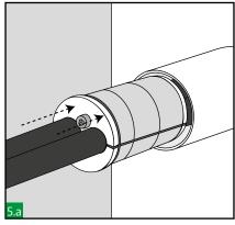
Insert the HRST into the sleeve.
