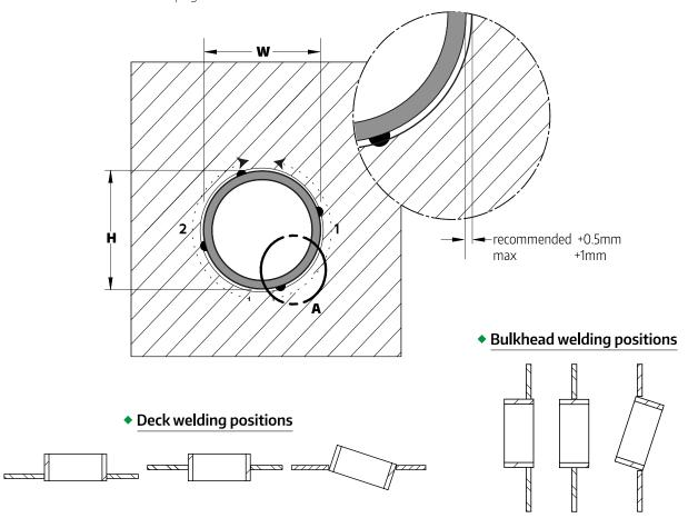
2. Tack weld on the front side, centring the frame onto the cut-out hole:
