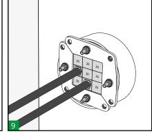
Tighten the nuts approximately 2mm each time following alternate tightening sequence, applying equal pressure to both plates. A minimum of 10 mm of thread should protrude on each bolt. Use a ratchet spanner for an easier installation.
