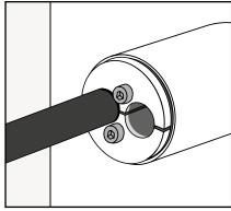
Check that every not occupied HRST holes are plugged with Hawke HRST plugs.
