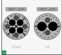
Tighten the bolts. Tightening must be done in one revolution step for each bolt following next sequence until the system is enough compressed to seal the cables.
