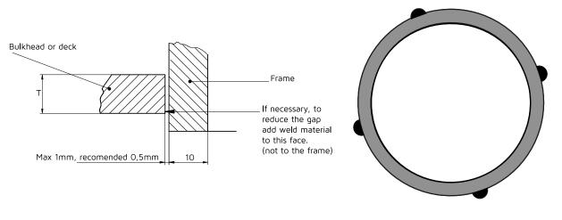
3. Start welding the frame with a sealing fillet weld on the backside. Follow appropriate welding sequence. This welding throat should not excess of 3mm.
