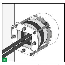
Extraction is achieved by releasing the compression, i.e. by reversing steps 7 and 8 and screwing M8 bolts (not supplied) into the threaded holes at each corner of the front plates. These releases the assembly from the aperture and allows the system to be disassembled.
