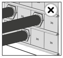
Check that there are a stayplate between each row of blocks and there are not stayplate between the bottom row of blocks and the frame. Check that all block are installed in position between the stayplates retention lips.
