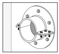
Check the inside diameter of the sleeve and the outside diameter of the cable/pipe to verify that it is within the range of selected HRST.
