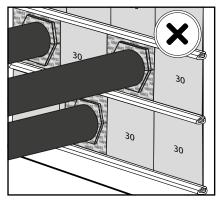
Check that there are a stayplate between each row of blocks and there are not stayplate between the bottom row of blocks and the frame. Check that all block are installed in position between the stayplates retention lips.
