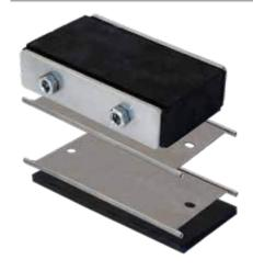
Hawke CSDM Compression system is used in H-DM frames to compress and seal the installation of cables and DM modules. It includes the endpacker unit, 5mm filler strip and two stayplates. The 5mm filler strip can be installed as either the top or bottom row of blocks within a H-DM aperture.
