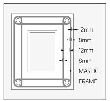
Cut nozzle on Mastic/Silicone tube to produce a bead diameter of approximately 8mm.
