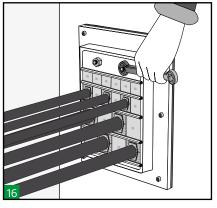
Tighten the nuts on the endpacker in alternate order to compress and complete the seal.
