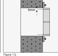
Size to fixing holes and type of fastener is to be established by the civil contractor dependent on size of frame weight and structure to which it is to be fixed. When fixing frames to concrete/brick type structure care should be taken if using expanding type fixings as they could
