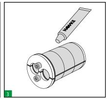
Lubricate the inside of the HRST to be in contact with the cables and lightly lubricate the outside in contact with the sleeve.
