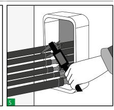
Take measures of cables diameters and select the appropriate Hawke tolerant blocks.
