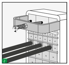
Remove endpacker nuts and front plate.
