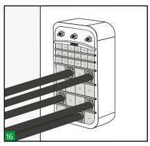
Make a visual inspection of the transit. Check that marks in all the cables are visible to be guarantee blocks and cable copper tapes are aligned.
