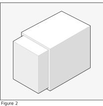
For hawke frames which are cast into a wall or floor it is recommended that a Hawke Polystyrene Mould is used. Hawke moulds are available to suit sizes 2, 4, 6 and 8 with 300mm lengths and may be cut to suit the deep of the wall or floor as required. (See catalogue page...79)
