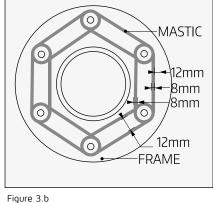
Cut nozzle on Mastic/Silicone tube to produce a bead diameter of approximately 8mm.
