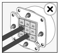
Check that there are sufficient blocks installed into the frame to cover the sealing area defined for each size of frame.
