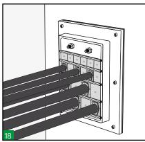
Make a visual inspection of the transit. Hawke's colour coding enables the installation to be visually inspected after completion and ensures correct matching of the blocks halves.
