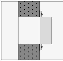
Size to fixing holes and type of fastener is to be established by the civil contractor dependent on size of sleeve weight and structure to which it is to be fixed.
