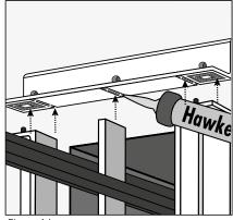
If HCOX open frame is used, Mastic/Silicone should be applied also in all bolting areas of the removable end as showed below.
