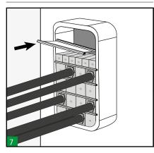
A stayplate is always inserted between each layer of blocks. Blocks should not protrude out of the stayplates retaining lips.
