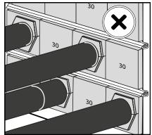
Check that Hawke Lubricant has been used during the installation.
