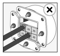
Check that stayplates have not be used in the installation.
