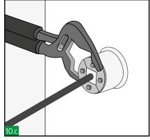
Slide the two front plates together and keep it fixed. Ensure all the blocks are located inside the front retaining lip. For an easier installation, cable ties, bolts or adjustable pliers can be used to close this plates.
