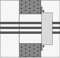
The sleeve can be bolted to wall and floors.
