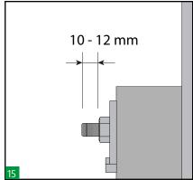
Approximately 10-12 mm of thread should protrude on each bolt to ensure the sealing.
