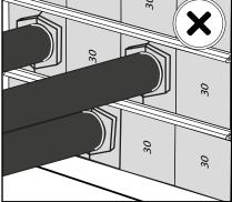
Check the correct orientation of the blocks.
