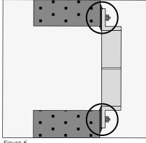
The frame can now be placed over its fixings and fasteners tightened to clamp the frame to the wall/floor.
