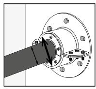
Check the inside diameter of the sleeve and the outside diameter of the cable/pipe to verify that it is within the range of selected HRST.
