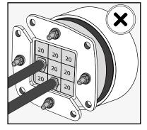
Check that the HRT/HRTO is completely inserted in the Sleeve/Aperture.
